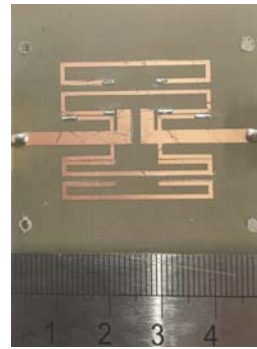
Substrate with \epsilon_r=2.6 and thickness t=1.0\text{mm}
